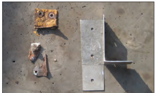
Remains of old bracket and new bracket
