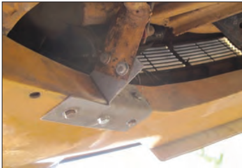
New bracket fitted
